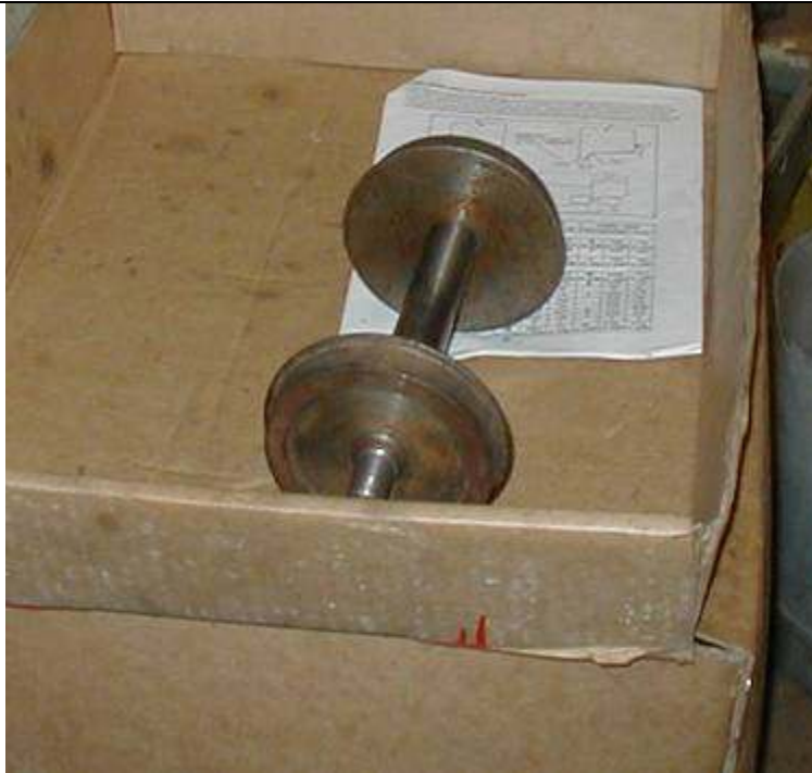
Wheels for the broken riding truck are pressed onto the axles.
