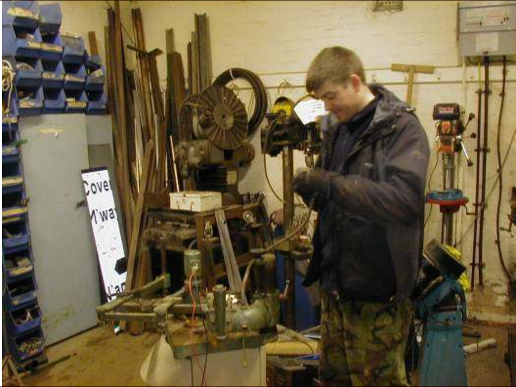
An engraving machine donated to the club failed its PAT test, Rob sets about locating the fault.
