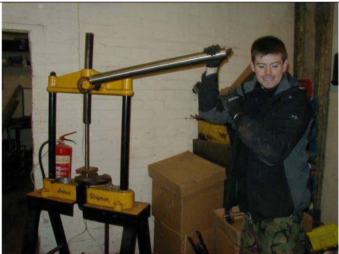
A slight measuring problem (oops) requires one of the wheels to be pressed back off.
