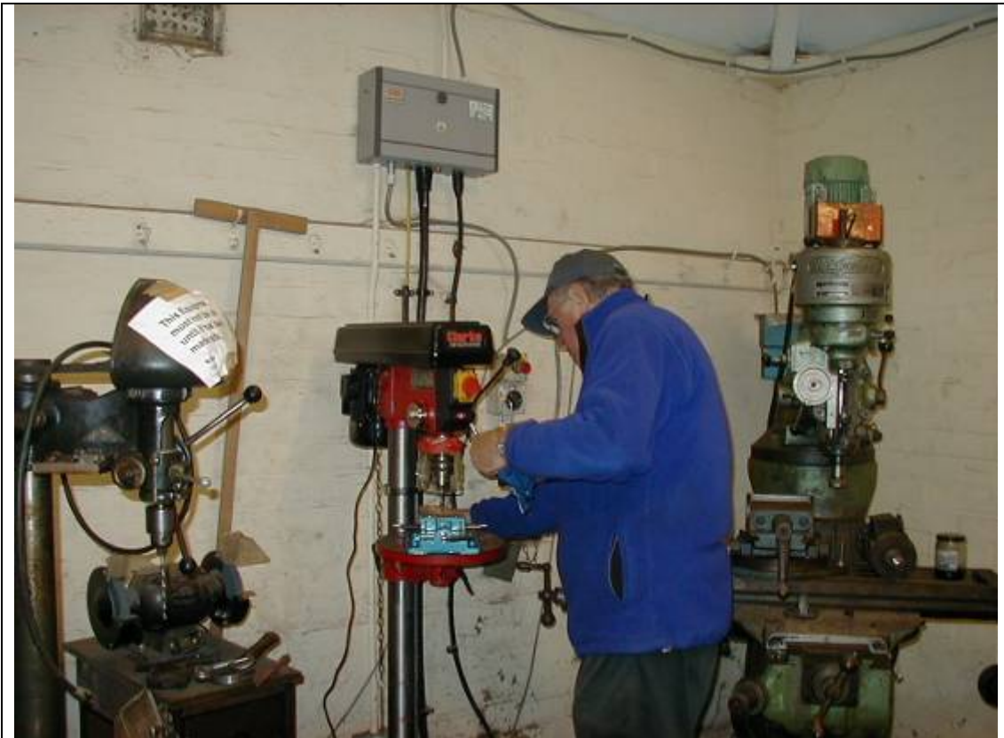
Chris fabricates new brake rods for the riding truck.
